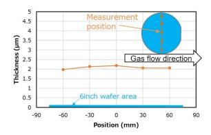
Fig. 3 Thickness distribution of β-Ga<sub>2</sub>O<sub>3</sub> film formed on a 6 inch test wafer
