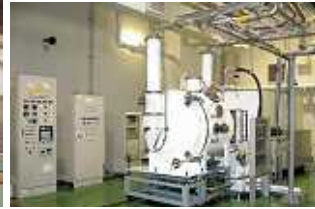
Inner-Planet Thermal Vacuum Environment Simulator, a compact space chamber
