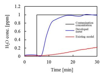
Fig. 2: Example of measurements of trace amounts of moisture in nitrogen
