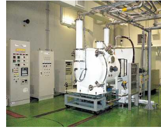
Small-scale space simulation chamber Used to test satellite components, engine endurance, etc.
