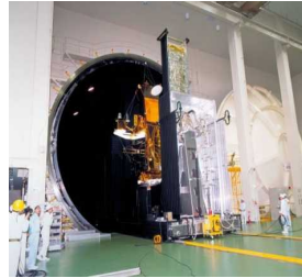
Large-scale space simulation chambers Used to test satellites
