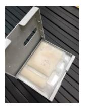
Fig. 1 25 cc cell cryopreservation bag
