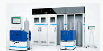
Gas cylinders weighing over 50 kg each are automatically delivered by a robot.
