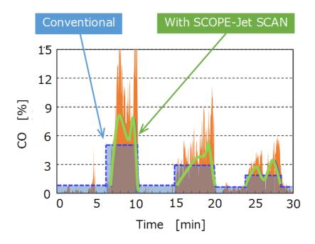
Fig. 2 SCOPE-Jet® SCAN controls the volume of oxygen flow
