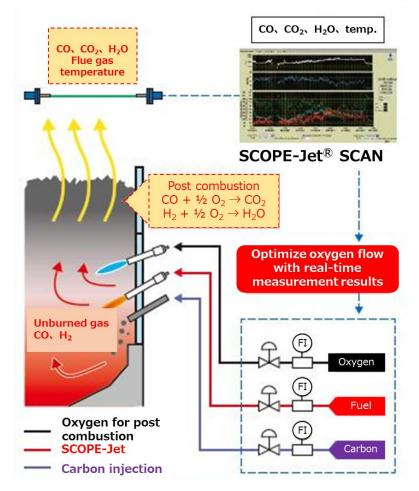
Fig. 1 SCOPE-Jet® SCAN system Overview
