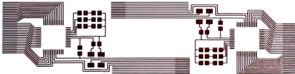
Fig. 2 Conductive wiring pattern made with copper nanoparticle ink printed using an ink jet printer
