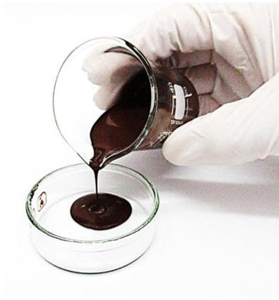
Fig. 1 Appearance of conductive ink
