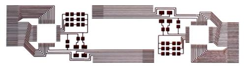
Fig. 2 Conductive wiring pattern made with copper nanoparticle ink printed using an ink jet printer
