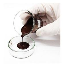
Fig. 1 Appearance of conductive ink
