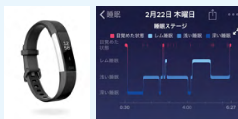
Alta-HR wristband-form wearable devices were distributed to employees. These devices enable individuals to monitor sleep quality (shown above), total daily activity (steps taken, distance covered, amount of time active, calories consumed) and other data.
