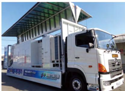
Hydro Shuttle mobile hydrogen station
