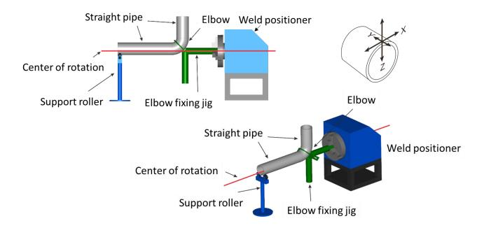
Fig. 3 Example of elbow fixing jig
