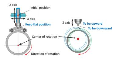
In conventional system the weld position change causes inconsistent welding results
