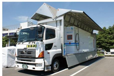
Hydro Shuttle® hydrogen refueling station mounted on a truck
