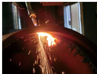
Cutting steel with Sun Cutter® HL-1
