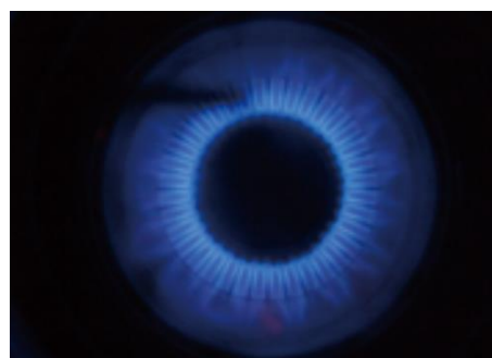
New compact combustion-type exhaust gas abatement system: Flames in burner
