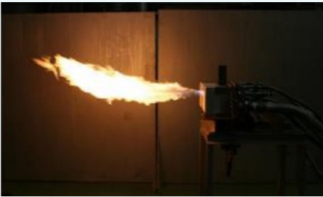
Innova-Jet® swing produces a flame that heats a wide area efficiently and uniformly using automated oscillation
