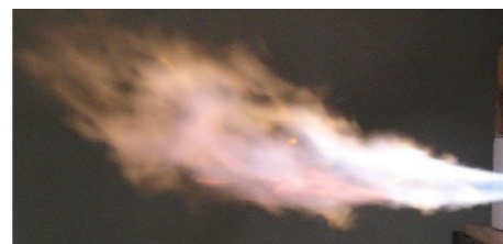
Flame from 100% hydrogen combustion
