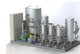
External view of the CO 2 capture system (Illustration)
