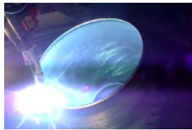
Metal AM fabrication process using the WAAM method
