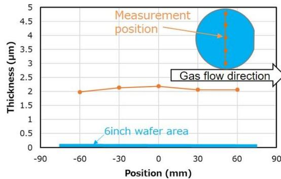
Fig. 3 Thickness distribution of  $\beta$ -Ga<sub>2</sub>O<sub>3</sub> film formed on a 6 inch test wafer
