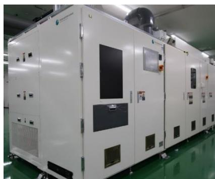
Fig. 2 Exterior view of the HVPE system of 6 inch single wafer for growing  $\beta$ -Ga<sub>2</sub>O<sub>3</sub> film
