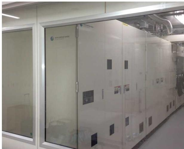
The MOCVD equipment made by TNSC (and installed in the Innovation Center) used in the joint research with world's largest processing capacity (yield rate of six eight-inch substrates)
