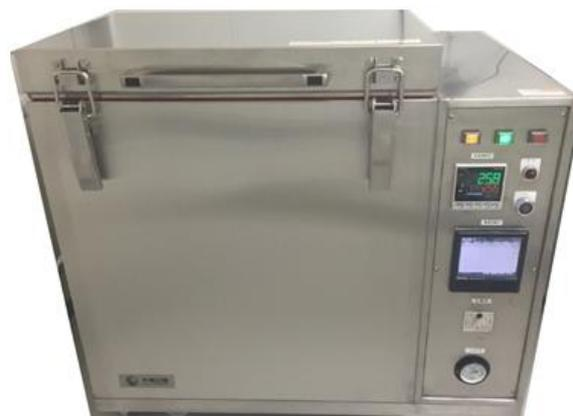
Fig. 2 CM-100 large-scale liquid nitrogen program freezer
