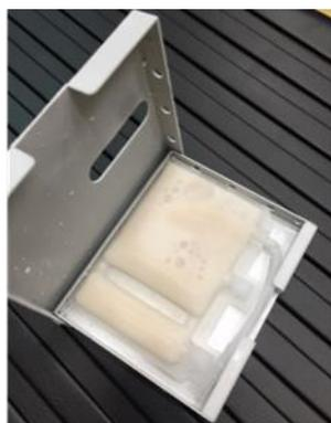
Fig. 1 25 cc cell cryopreservation bag
