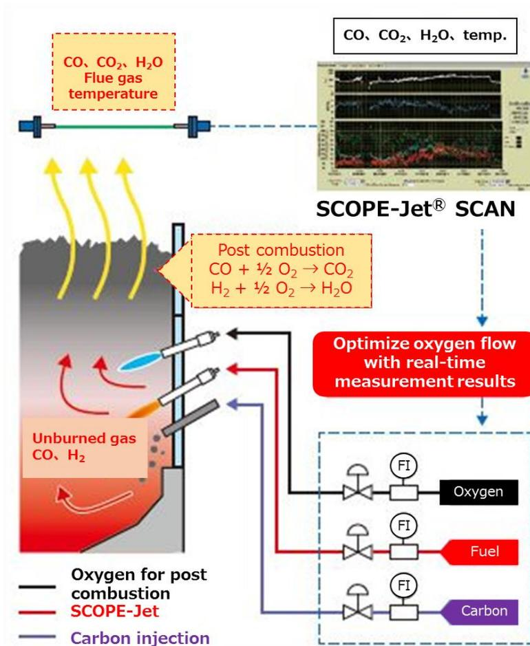
Fig. 1 SCOPE-Jet® SCAN system Overview
