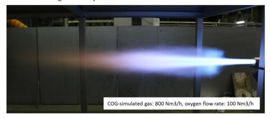
(COG-simulated gas composition: CH4: 45.7%, C2H6: 2.7%, C3H8: 2.2%, C4H10: 1.0%, N2: 48.4% Low calorific value: 19 MJ/Nm3)
